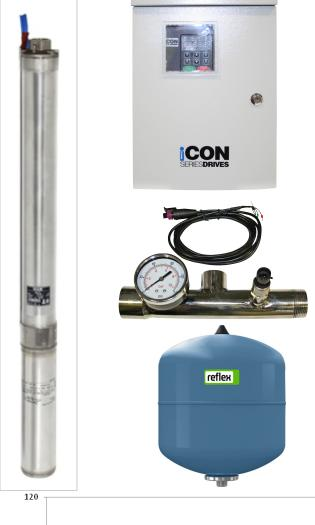
The iSUB22 device supplied with BIA-ISUBS4B16M, is an innovative 240V single phase input built-in variable speed control system housed in a weather proof fan ventilated enclosure and incorporates a manifold with pressure gauge and pressure transducer for easy installation.
